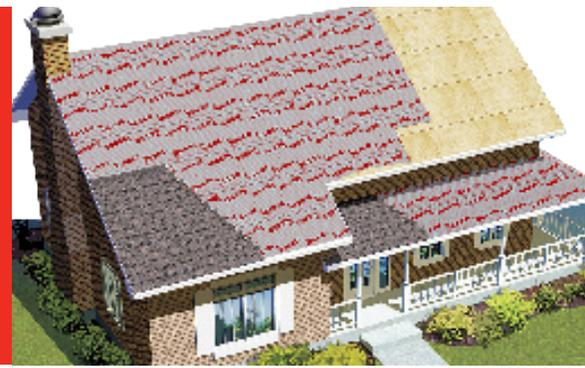
Lightweight synthetic underlayment which has a very high tensile and tear strength allowing it to be used as a temporary coating for exposed roofs. In addition, it replaces asphalt felt boards.
