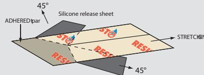
4. While applying pressure to the other end of the membrane, press the membrane to the support with a scrub brush by pressing from the center toward the sides of the membrane.
