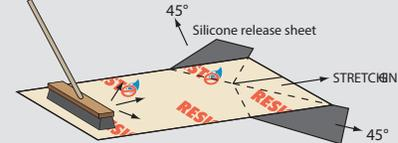
5. Continue to remove the protective film while applying pressure with the broom on the bonded portion.
