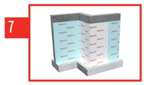
Install the full pieces of membrane, and make sure that they completely cover the joints and the ends of the reinforcement pieces.
