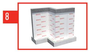
It is recommended to mechanically fasten the top termination of the membrane with a termination bar.
